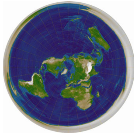
Inverse exponential map of the earth at the north pole, namely an equidistant azimuthal projection.
